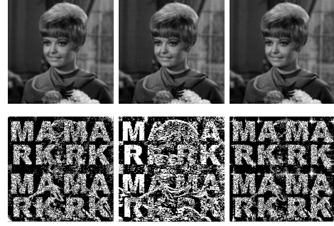
Figure 1: Watermarked image (upper row) and extracted watermark (lower row)
