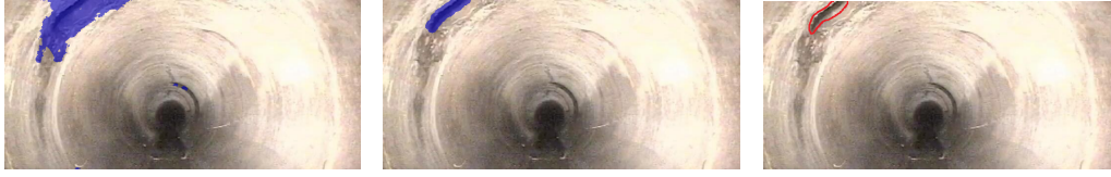
Figure 2: Example of detection results (Left:SegNet, Center:Proposed Method(SVM), Right:Ground-truth defect label)
