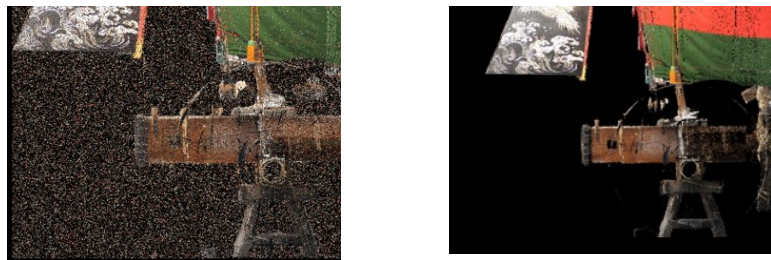
Fig.4 Left: 3D scanned point with outlier noise added. Right: Result of the proposed method.
