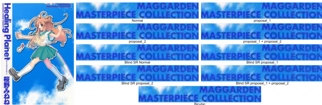
Fig2. Manga109 HealingPlanet x4 (Degraded image saved 10 times with jpeg quality 30)
